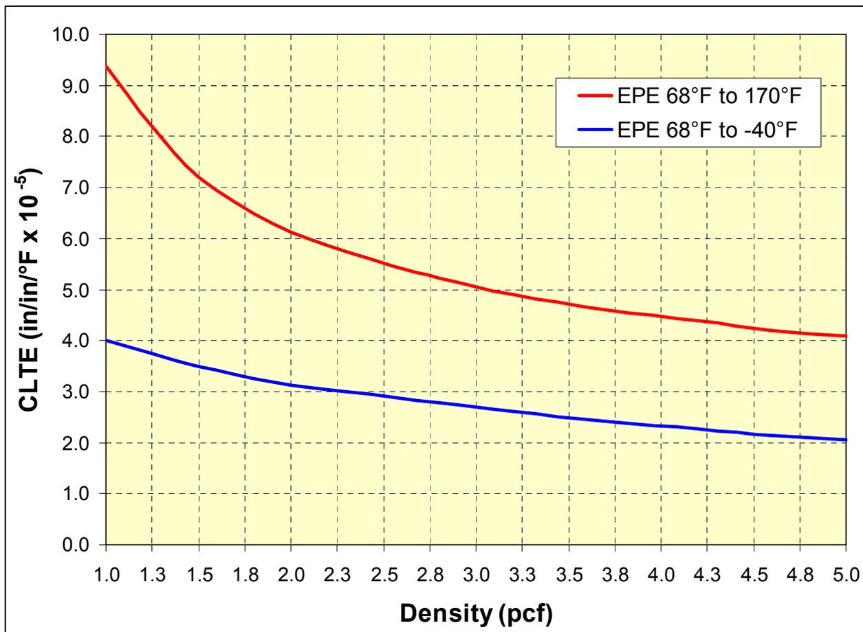
Note: Tested per ASTM-D696
