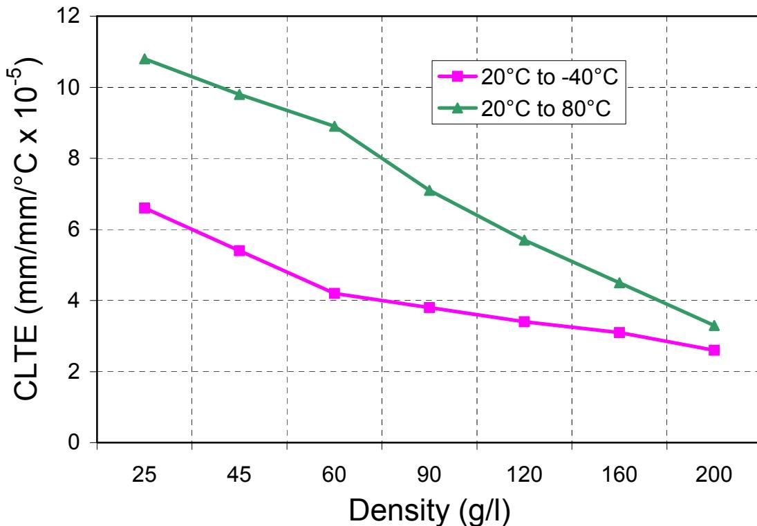
Note: Tested per ASTM-D696
